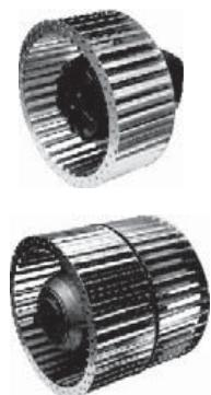
The impellers with 38-42 forward curved blades are made of galvanized sheet metal. They are mounted directly to the external rotor motor.
